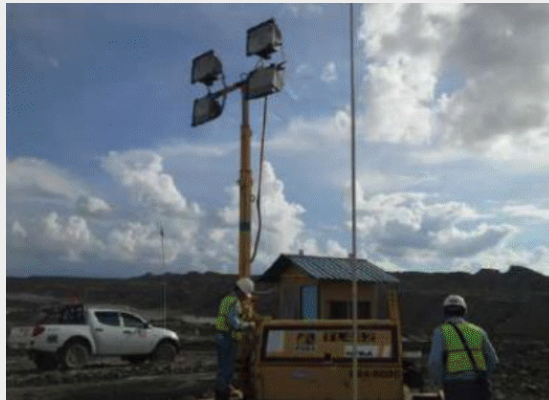
Mobile Tower Lamp, 1500W Metal Halide vs LED Power Spot 300W & 500W
