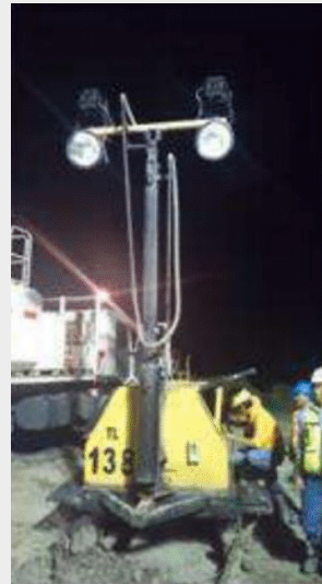
Mobile Tower Lamp, 1500W Metal Halide vs LED Power Spot 300W & 500W
